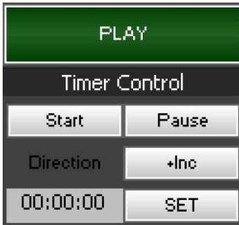
There is a *Timer Control* menu which appears under the **PLAY** button on right side of *Work area*. The **Start** and **Pause** buttons are used for starting or pausing the **Timer** object which currently runs on air. - **Dec** sets the object as countdown timer, and **+Inc** sets the object as count up timer; in **Direction** under *Timer Control* menu. You can set an initial time by pressing the **SET** button.
